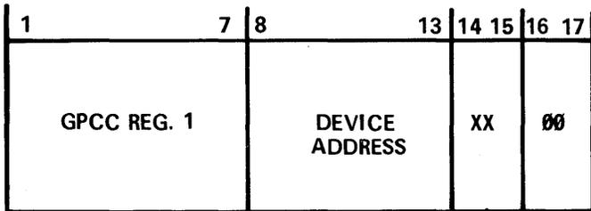
ZERO – SET BY GPCC HARDWARE TO CREATE WORD BOUNDARY MACHINE ADDRESS
