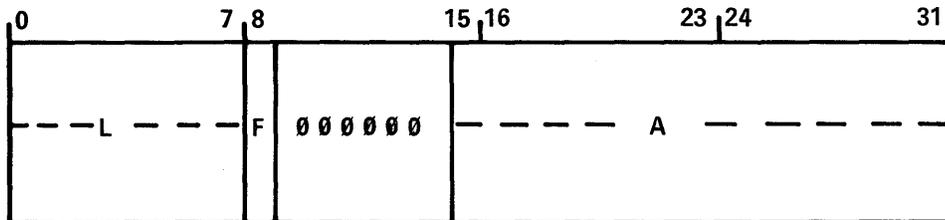
ADDRESS OF STORAGE WHERE TRANSFER WILL BEGIN; WILL BE INCREMENTED BY 1 UPON TRANSFER OF ONE BYTE.
