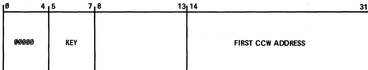
SPECIFIES THE DOUBLE-WORD STORAGE LOCATION WHICH CONTAINS THE FIRST CCW IN THE CHANNEL PROGRAM OR THE CSW ADDRESS (ONLY LEAST SIGNIFICANT 18-BITS UTILIZED)
