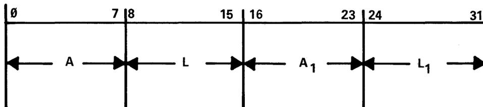
WHEN THE L-FIELD OF THIS WORD IS DECREMENTED TO ZERO THE BITS 16 THRU 31 REPLACE BITS 0 THRU 15; NO HARDWARE MODIFICATION IS DONE ON A<sub>1</sub> OR L<sub>1</sub>.
