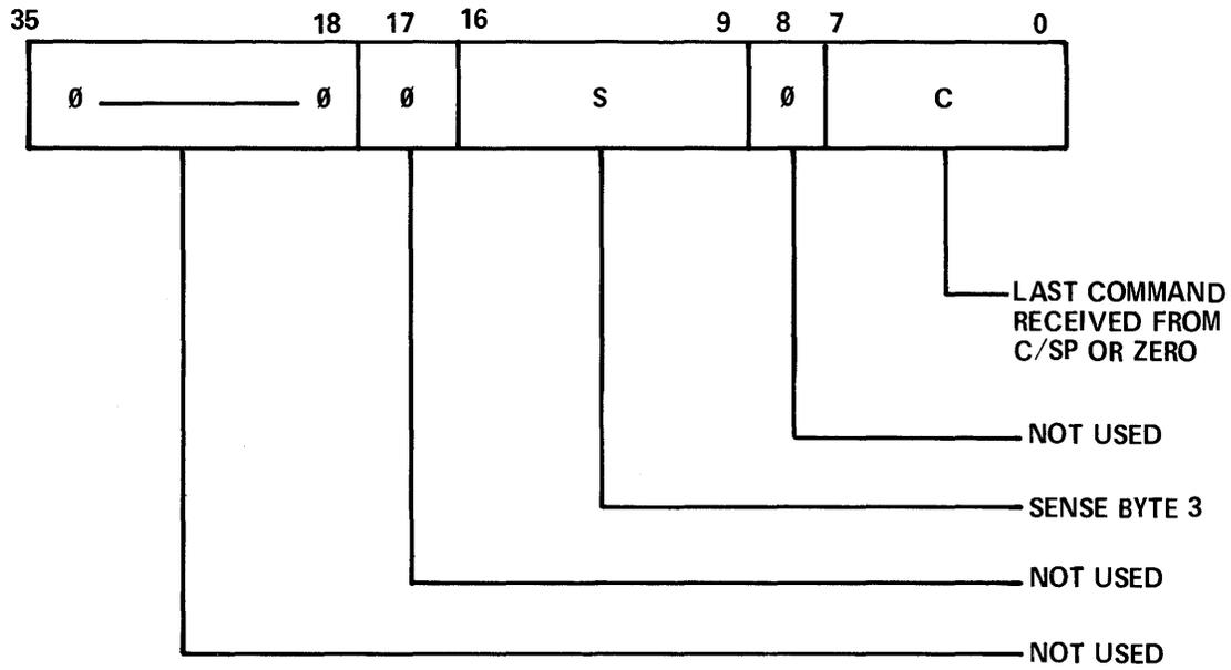
THE S AND C PORTIONS OF THIS WORD WILL BE ZEROED DURING THE ENDING OF THE INTERRUPT SEQUENCE.
