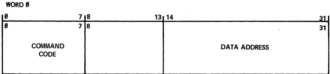
STORAGE ADDRESS OF THE FIRST BYTE OF DATA TO BE TRANSFERRED, UNLESS COMMAND CODE IS TEST I/O OR TRANSFER IN CHANNEL, THEN THIS FIELD IS ADDRESS OF NEW CCW (ONLY 18-BITS MAY BE UTILIZED)
